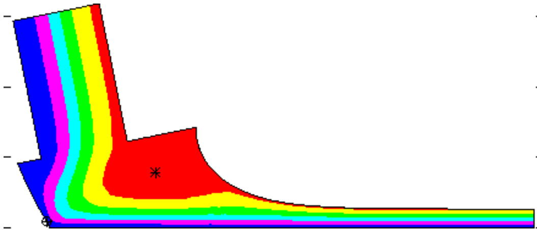
Figure 11. Stream Function for optimal design at Gap=0.035 cm, \alpha=0.2 rad (cost=300)
